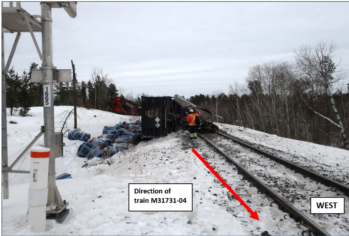
Figure 2. Nickel sulphide bags spilled from first derailed car (Source: TSB)
