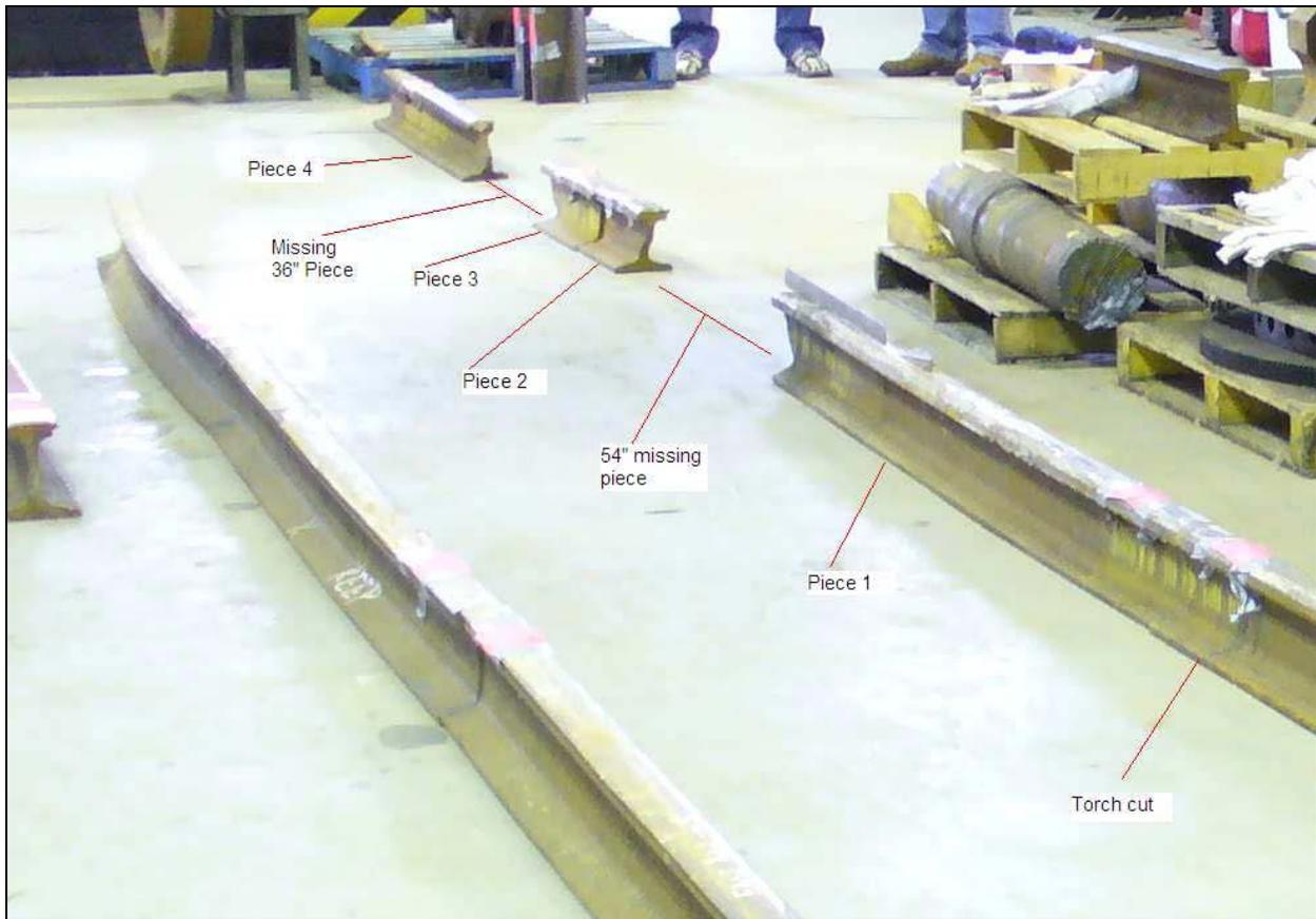
**Photo 1.** Layout of the east rail (left) and the west rail (right)
