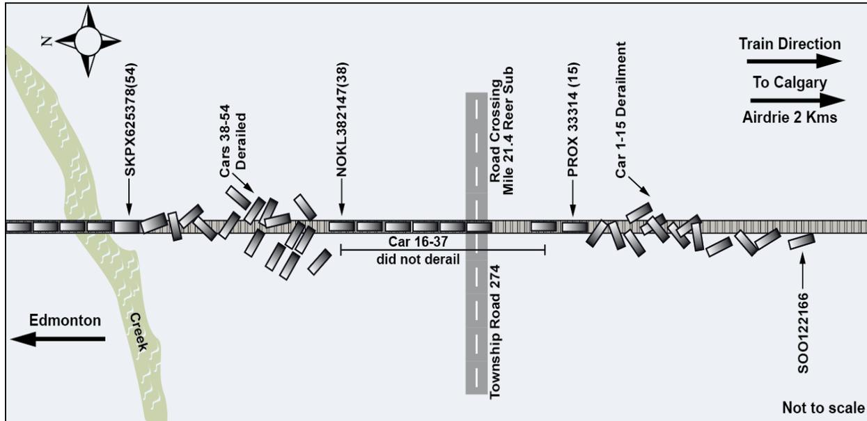
Figure 2. Derailment Site Diagram
