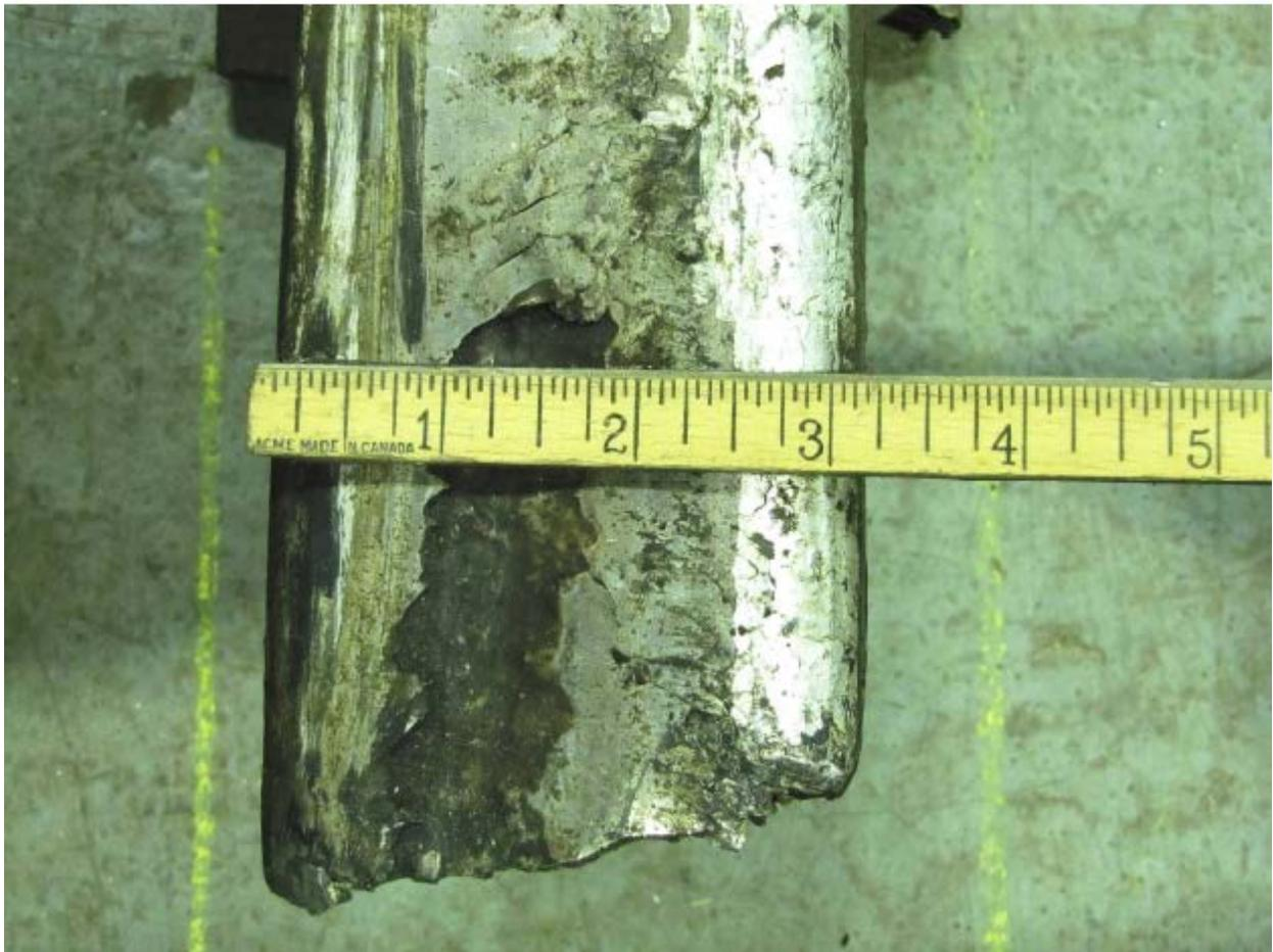
**Photos 2 and 3.** Fracture at the south end of the 3 mating west rail pieces showing material flow and heavy checking on the gauge corner. A 10 inch long section of rail head was crushed measuring approximately 7/16 inches at it deepest point. Corresponding shelling was also observed on the running surface at the fractured south end.
