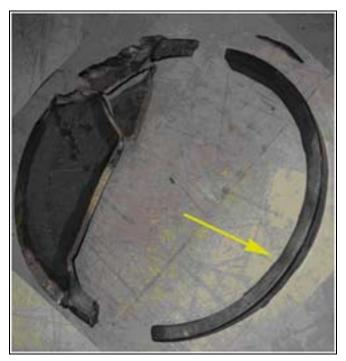
**Photo 1a.** The Yellow arrow points to portion of broken wheel recovered at Mile 0.6 of the Dundas Subdivision.
