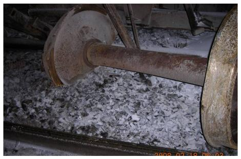
**Photo 3**. Straight-plate wheel set with one broken wheel at site of derailed cars
