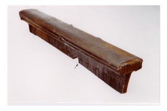
The second piece of rail was found to have a vertical fracture and a longitudinal fracture, which was a continuation of the fracture observed in the first piece. The longitudinal fracture was flat and free of chevron markings, consistent with progressive cracking. The surface of the vertical fracture had chevron markings pointing towards the middle of the web. There was little damage due to wheel pounding on the head fracture surfaces.
