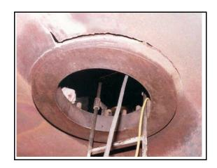
analysis determined that the impact on the tank car nozzle was several times greater than that required to exceed the design strength of the car structure.
