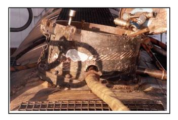
gradually, which prevented the formation of a large cloud of gas at the time of the occurrence. Liquid ammonia was still slowly leaking from the car 24 hours after the occurrence.
