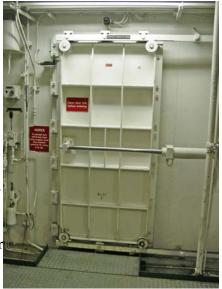
The doors are typically operated in the manual mode when the vessel is secured alongside. In this mode, the doors are opened and closed locally by actuating the operating lever; but when the lever is released, the door movement stops and it remains in that position, at the point the lever was released.
