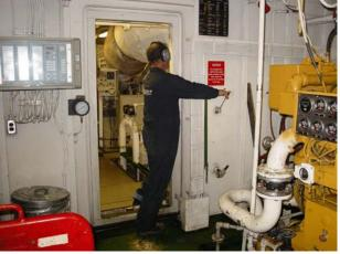
In the case of the two vertical sliding watertight doors, the axis of rotation for the operating levers was 37 cm and was, therefore, closer to the edge of the door. However, access to the operating levers on one side of both doors was restricted by an angle frame (see photo 6). Additionally, the lever operation of the two doors was not consistent. In one case, the door was opened by pushing the lever, while in the second case the lever was pulled.
