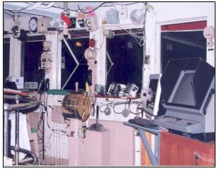
**Photo 3.** The pilot's seat is located between the controls on the left and the ECS on the right.
