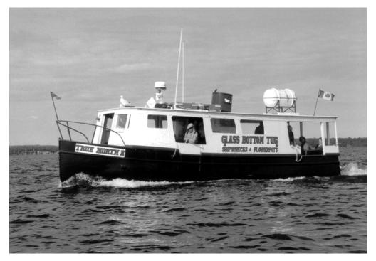
The wooden superstructure, which provides shelter from the weather for deck passengers, is open at the after end and has large passenger embarkation openings in the port and starboard sides forward of midships.
