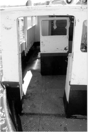
Reinforcement or repairs to the bridge front included the fitting of an additional layer of plywood over the original structure installed when the vessel was converted to passenger service. The inner layer of plywood was in a deteriorated condition due to dampness and rot, and several voids had developed between the layers where the inner layer had disintegrated.
