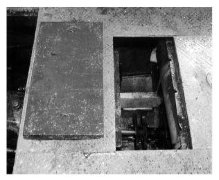
Main deck plating was extensively corroded around the boundary of an irregularly shaped opening that provided access to the main engine control, steering gear and electrical cables inside the wooden console at the steering position. This opening allowed any water shipped and retained on the main deck to freely enter the underdeck compartment.
