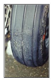
uncured state. The increase in stopping distance as a result of hydroplaning is impossible to predict accurately, but it has been estimated to increase by as much as 700 per cent. Performance graphs for the aircraft indicate that a landing distance of 4 400 feet was required for the aircraft at the calculated landing weight of 22 198 pounds. Landing distance was calculated for a bare, dry runway condition.
