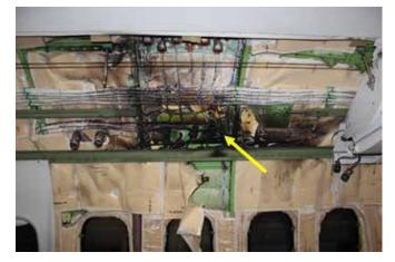
The electrical arcing that occurred before the 50 A thermal-type circuit breaker tripped caused minor pitting damage to adjacent wiring bundles, and heat damage and sooting to the insulation blankets and the structure of the outer panel of the overhead baggage compartment(Figure 2 and Figure 3).
