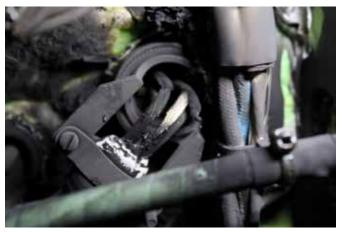
In both events, the connectors were found to be heat-damaged. In 1 of the occurrences, the damaged connector was located in an engine nacelle AC control box, and in the other occurrence, connector 9811-J711 was damaged. Bombardier conducted its own investigation into these 2 occurrences and determined the following:
