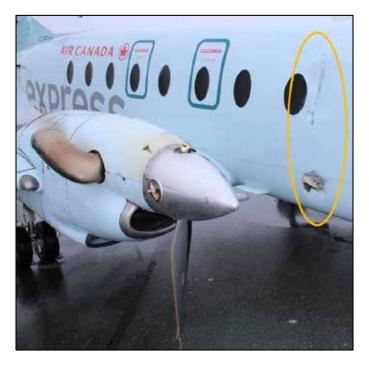
The upper dent caused the window interior trim and cabin interior to fracture and come loose inside the cabin. A portion of blade penetrated the cabin wall just above the floor level between seats 1B and 2B. About 19 inches of the blade tip remained embedded (Figure 4).
