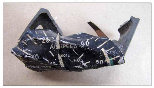
Photo 1. Occurrence airspeed indicator showing trapped pointer position
