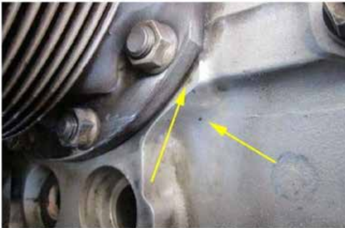
Figure 1 - Failure of a weld-repaired crankcase. Note crack from the cylinder base stud.
