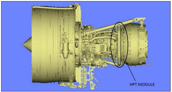
Figure 1. Location of the HPT module on the engine
