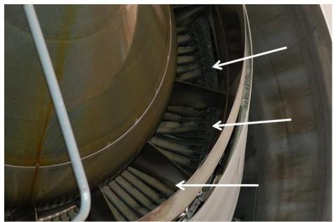
Photo 1. LPT blade damage at the aft end of the engine
