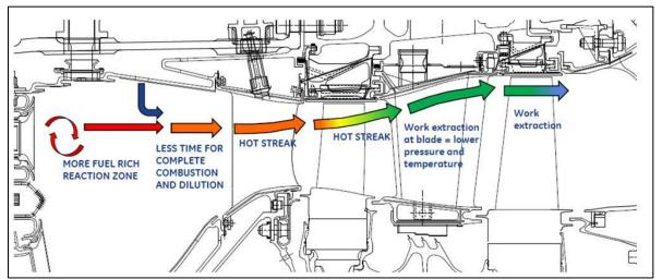
**Figure 2.** Diagram shows fuel rich area, and coloured arrows show the gas flow through the HPT stages in the engine (Source: General Electric)
