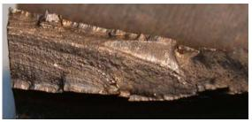
Photo 1. Fractured 3rd stage compressor airfoil
