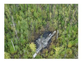
All major components of the aircraft were located at the accident site. No discrepancies were found with the portions of the aircraft that could be examined. Only small fragments of the windshield were found within and immediately outside of the site perimeter.
