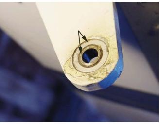
used to measure the force required to rotate the clevis; the results averaged 52.7 pounds of force. It was noted during the tests that the inner bushing remained fixed in the outer bushing and the clevis rotated about the inner bushing (see Photo 2). The clevis is designed to remain fixed to and rotate with the inner bushing.
