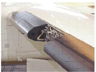
Photo 1. Missing number 4, left, leading-edge panel
