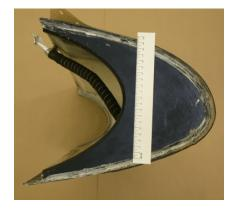
**Photo 2.** Cross-section of the left leading edge
