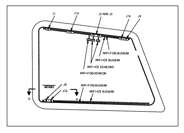
J1, J4, J1, J13, J15: Power TerminalsJ2, J3, J14: Sensor TerminalsNote: J13 and J15 are Anti-Fog (back-up) Power Terminals
