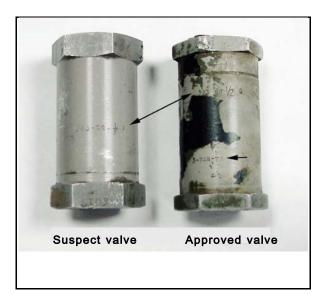
approved P/N 3-744-75 valve was measured at 132 cc/min with the flow beginning at approximately 4 inches of solvent. The flow rate for the non-approved valve was measured at 36 cc/min with the flow eventually beginning at 5 inches of solvent, after waiting a few seconds.
