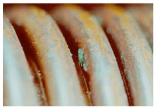
represented a difference in the bellows length of 0.0796 inches, which was much greater than the 0.007 inches allowed. The increased length was indicative of a loss of vacuum in the acceleration bellows. Also, there were a few portions of the bellows with very small patches of greenish-blue discolourations. These discoloured patches could be seen with the naked eye (see Figure 1). Thus, further technical investigation was carried out on the bellows.
