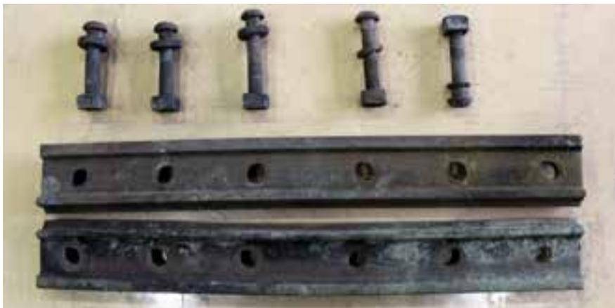
Figure 5: Joint bars and bolts connecting the heel rail with the frog rail
