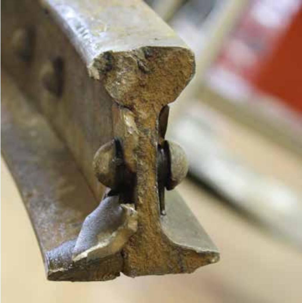
Figure 12: Fracture surface of the LH 22-foot switch point (location C in Figure 8)
