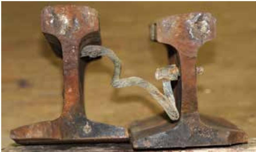
Figure 4: Fracture surfaces of the LH heel rail
