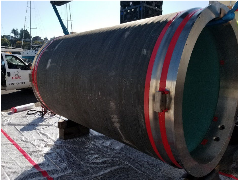
Figure 13. Full-scale cylinder with titanium rings from first construction of the Titan (Source: Patrick Loomis)
