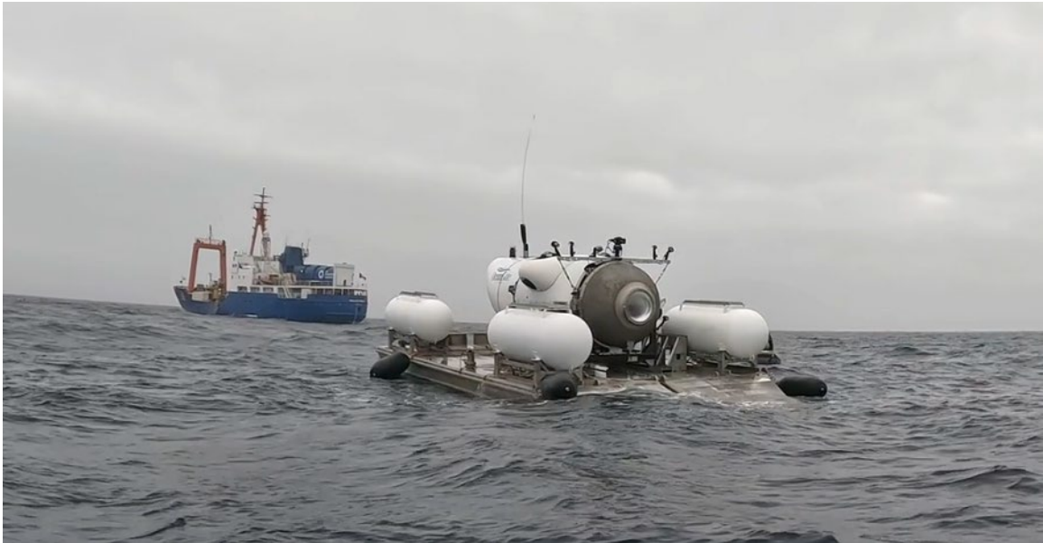
Figure 18. The Polar Prince towing the LARS and the Titan (Source: OceanGate)
