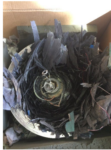
Figure 12. Carbon fibre end dome after test (Source: Patrick Loomis)
