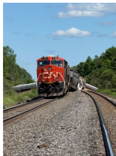
Figure 2. View of tail-end locomotive and derailed cars (Source: Canadian National Railway Company)
