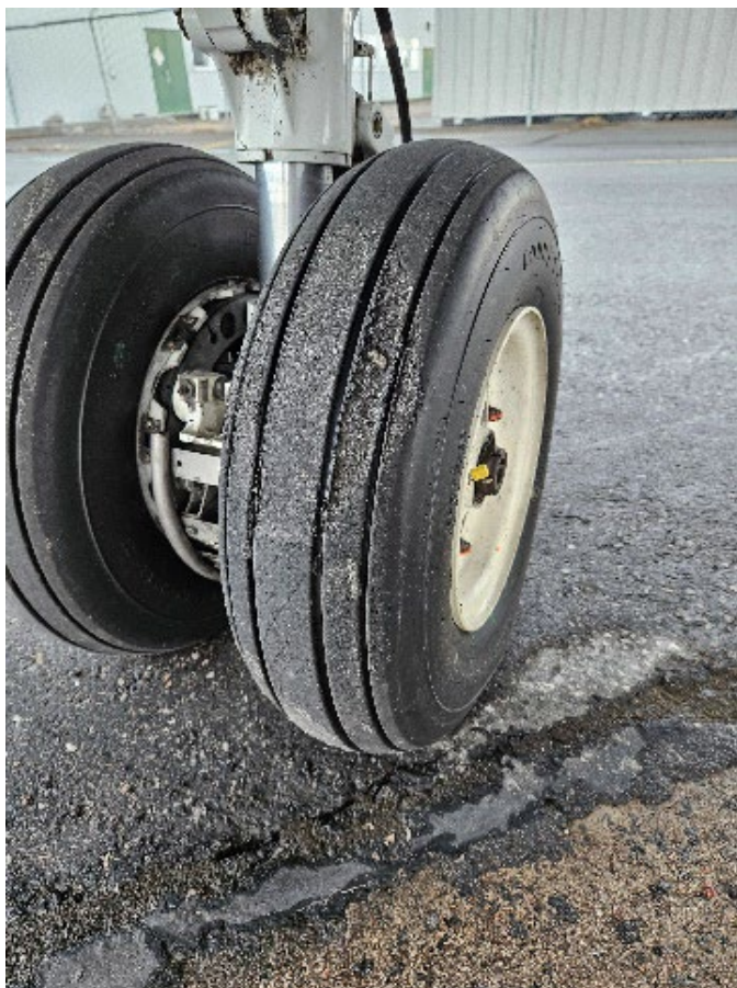
Figure 3. Reverted rubber on one of the occurrence aircraft's tires (Source: TSB)
