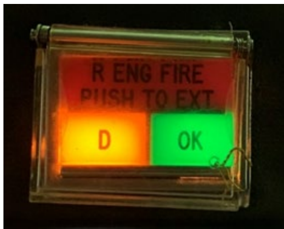
Figure 4. Occurrence aircraft's right-engine fire extinguisher control switch (Source: Keewatin Air LP)
