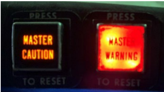
Figure 7. Occurrence aircraft's illuminated MASTER WARNING flasher on the right side of the warning annunciator panel (Source: Keewatin Air LP)
