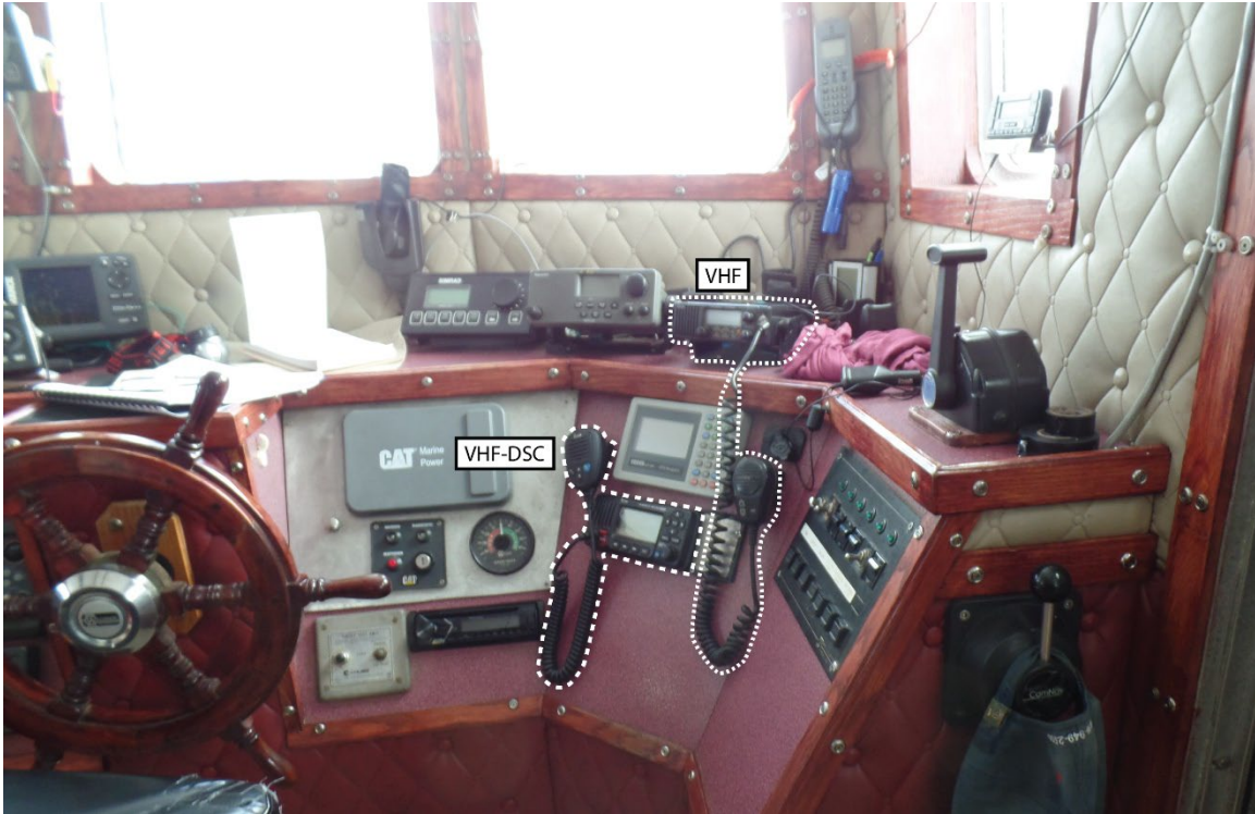
Figure 4. The Silver Condor's navigation console, showing the vessel's helm, propulsion control, navigation equipment, and radio equipment (Source: Third party, with permission and TSB annotations)
