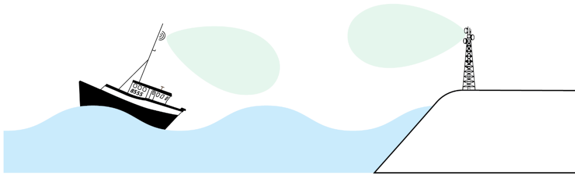
Figure 11. Diagram showing vessel and shore-based antennas misaligned in heavy seas (Source: TSB)
