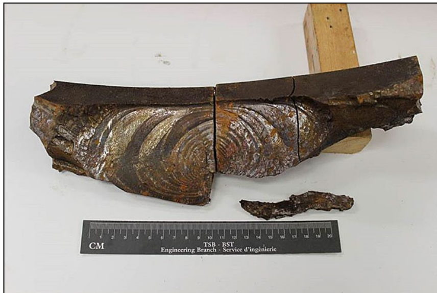
Photo 3. Shattered rim of L3 wheel
