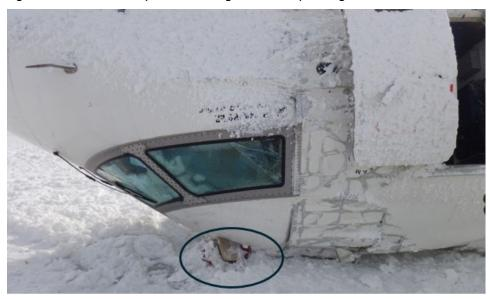
Figure 9. Location of escape hatch through which the pilots egressed (Source: TSB)
