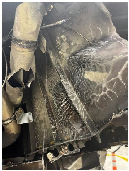
Figure 7. Close-up view of the thermal damage to the right wing (Source: TSB)
