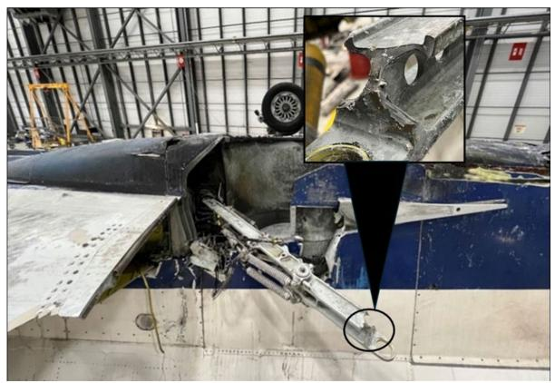
Figure 5. Occurrence aircraft resting inverted showing a close-up view of the fractured right main landing gear side-stay (Source: TSB)
