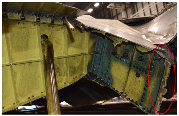
Figure 6. Right-wing rear spar, with fractured area (Source: TSB)
