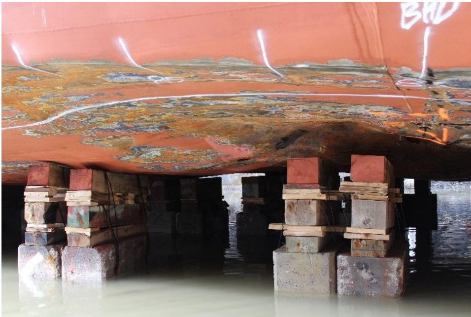
Figure 9. View of hull bottom shell plating deflections, breaches, and temporary repairs carried out by the divers off the Astronomical Society Islands (Source: TSB)
