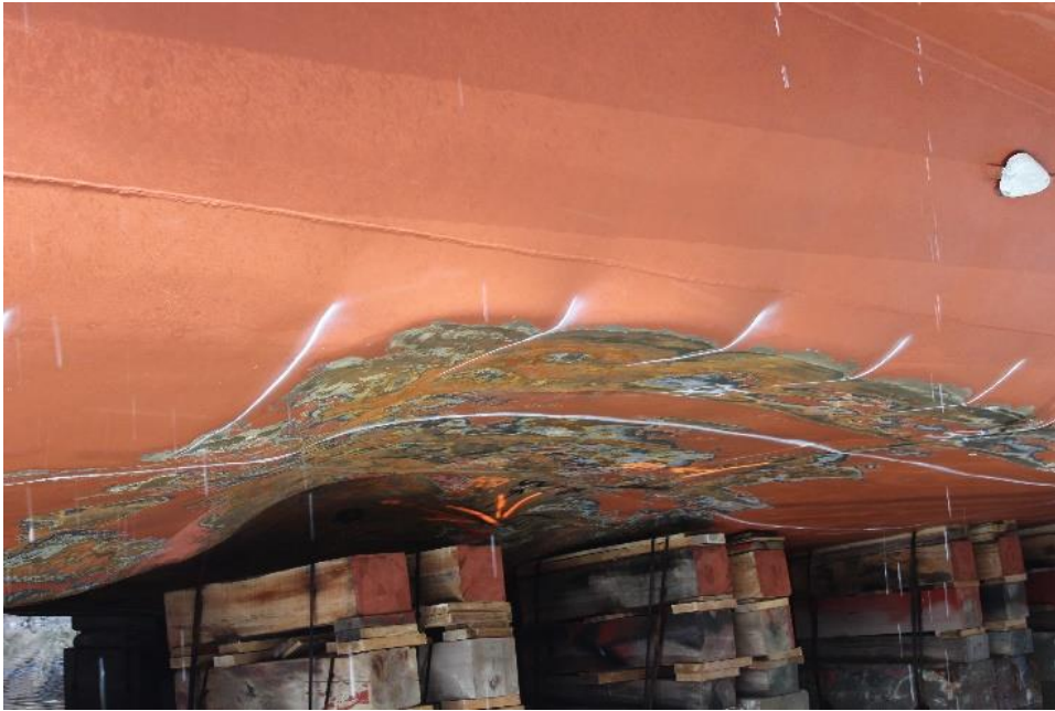
Figure 10. View of hull bottom shell plating deflections, breaches, and temporary repairs carried out by the divers off the Astronomical Society Islands (Source: TSB)
